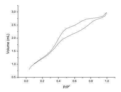
Figure 5. N<sub>2</sub> adsorption-desorption of mesoporous silica.
