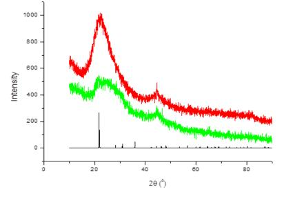
Figure 1. XRD pattern of (a) mesoporous silica (b) grafted catalyst.
