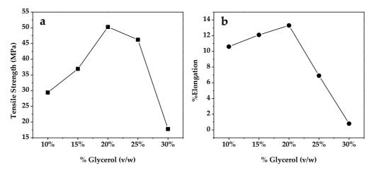
**Figure 2.** Mechanical properties of *Durio zibethinus* Murr starch-based bioplastic a) tensile strength and b) elongation, with various concentration of glycerol.
