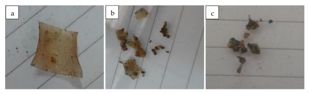
**Figure 5.** *Durio zibethinus* Murr starch-based bioplastic biodegradation test on soil a) day-0, b) day-5, c) day-7.
