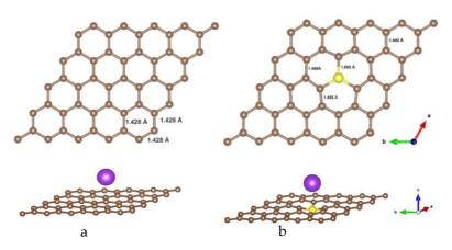
**Figure 1.** The 4x4x1 unit cell of (a) pure graphene and K/graphene, and (b) S-graphene and K/S-graphene. Brown, yellow, and magenta correspond to carbon, sulfur, and potassium ion, respectively
