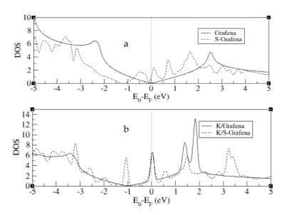
**Figure 3.** DOS after the Fermi level was set up into zero from (a) graphene and S-graphene, and b) K/graphene and K/S-graphene
