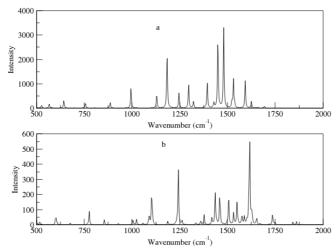
Figure 2. The wavenumber vibration of (a) Pure graphene and (b) S-graphene
