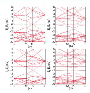
**Figure 4.** Structure of the band energy of (a) graphene, (b) S-Graphene, (c) K/Graphene, and (d) K/S-Graphene
