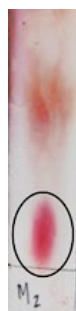
Figure 2. Polypeptide antibiotics determination in the methanol fraction after staining with 3% ninhydrin. The eluent system for TLC separation was a mixture of n-butanol: acetic acid: distilled water (3:1:1 v/v/v).
