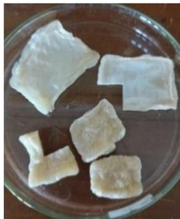
**Gambar 3.** *Solid Polymer Electrolyte* (SPE)
