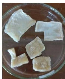
**Gambar 3.** *Solid Polymer Electrolyte* (SPE)
