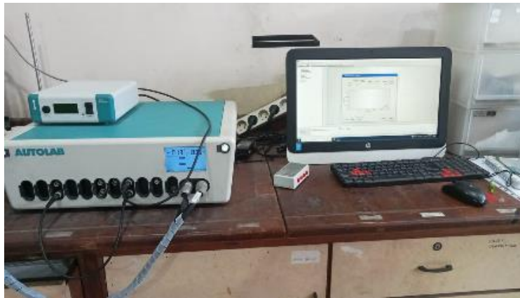
Figure 8. Corrosion Rate Testing Using a Potentiostat.
