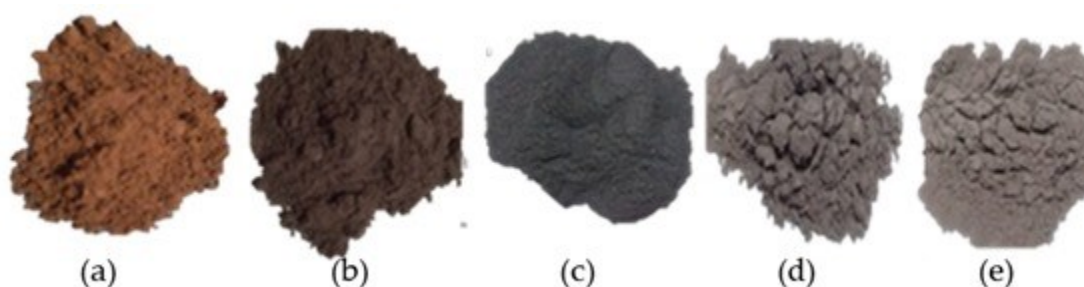
Figure 1. Photo of the synthesized samples of (a) \text{CdFe}_2\text{O}_4 , (b) \text{NiFe}_2\text{O}_4 , and \text{Ni}_{1-x}\text{Cd}_x\text{Fe}_2\text{O}_4 ( x=0.1-0.2 )
